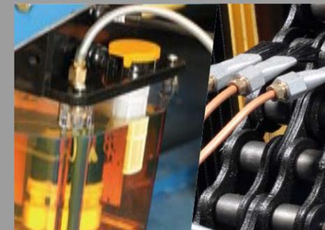
Automatic lubrication device
